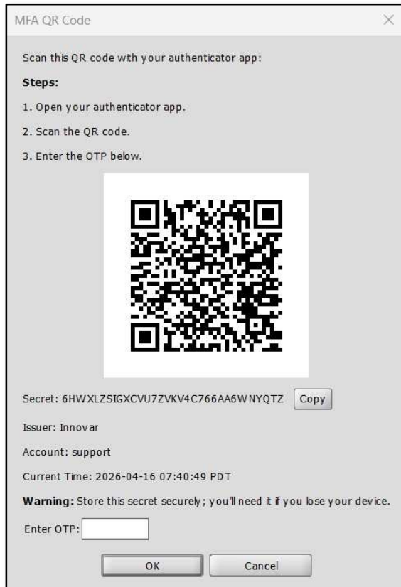
Figure 11: The MFA QR Code dialog showing the QR code, secret key, and OTP entry field.
